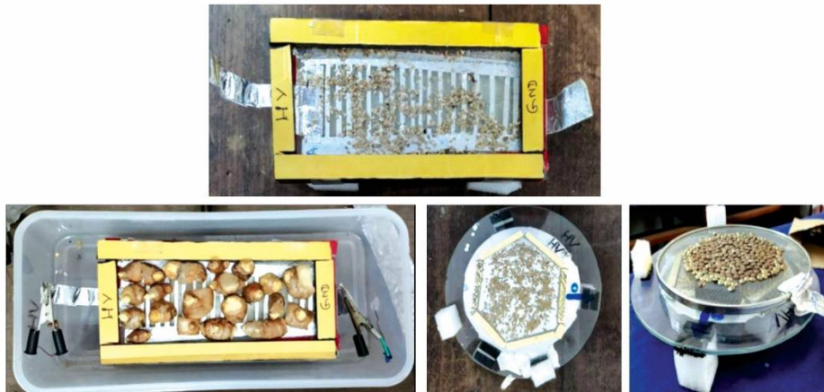
Fig. 5. Surface dielectric barrier discharge for tomato seeds, volume dielectric barrier discharge for tomato seeds, surface dielectric barrier discharge for ginger rhizome.
